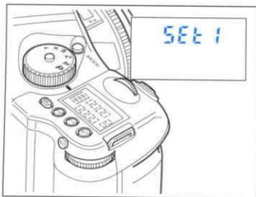
1. Set the shutter release mode selector lever to "S" (to turn the power on).
