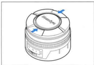
Grasp the lens front cap ring and remove.
